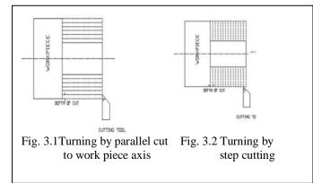
As solid cutting tool is used in microturning can produce the definite 3D shapes. In order to accurately and precisely control the cutting tool motions during machining, cutting path generation by computer programming is employed.
