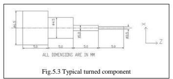
The first digit in each row indicates the block numbers. In '0' block, the initial diameter of the bar and the machining length is specified. In '1' block, the largest diameter of bar to be machined and its machining length is specified. In '2' block, the next largest diameter and the machining length of that diameter is specified. Like these blocks are specified and these files are saved in '.txt' format. The next step is importing this file to 'SLICER'.
